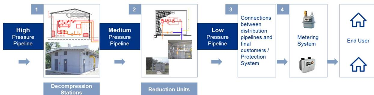
As at 31 December 2019, the system consists of 1,229 decompression and measurement stations (city gates) where gas filtration, preheating, reduction of pressure, measurement and odourisation are performed. City gates are the break points between transportation and distribution infrastructure systems. 2iRG’s stations are remotely measured and controlled.
